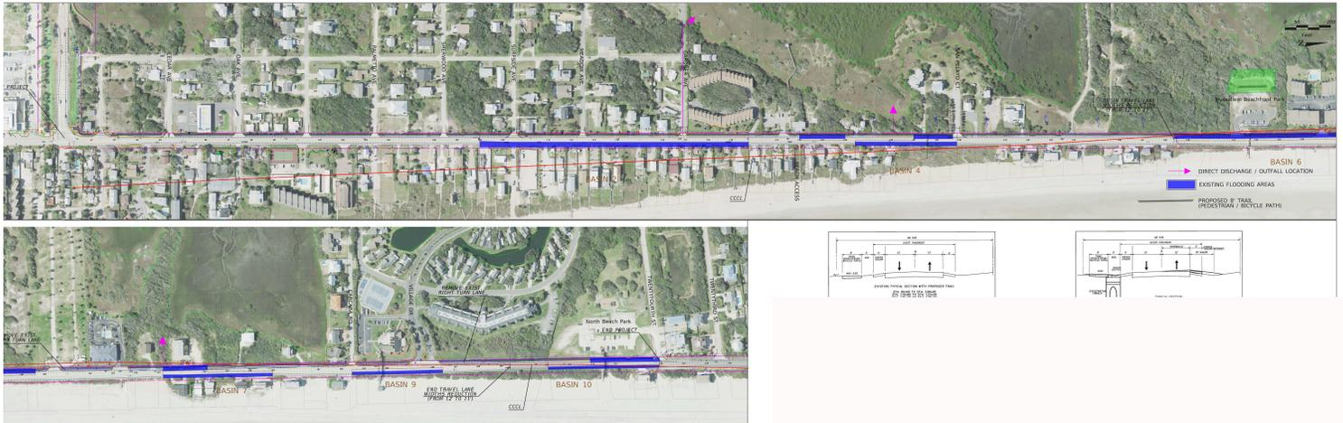
The above rendering represents the proposed 8-foot trail and drainage improvements to Coastal Highway from the State Road A1A intersection to 24th Street to reduce roadway flooding.
